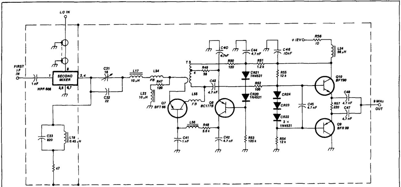
fig. 8. Second mixer of a receiver chain, including the diplexer, low-noise amplifiers, and power-output stage.
