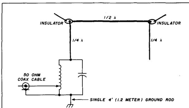
fig. 1. General arrangement of the half-square antenna, which originally appeared in *QST* and later in reference 1. It was described in these publications by Ben Vester, K3BC.
