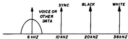
fig. 1. Proposed spectrum arrangement for the MSTV fm system.
