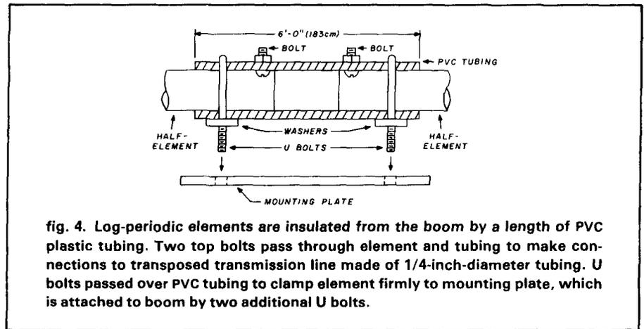
fig. 4. Log-periodic elements are insulated from the boom by a length of PVC plastic tubing. Two top bolts pass through element and tubing to make connections to transposed transmission line made of 1/4-inch-diameter tubing. U bolts passed over PVC tubing to clamp element firmly to mounting plate, which is attached to boom by two additional U bolts.
