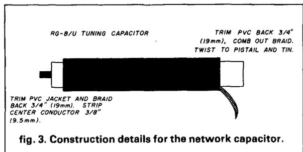
fig. 3. Construction details for the network capacitor.
