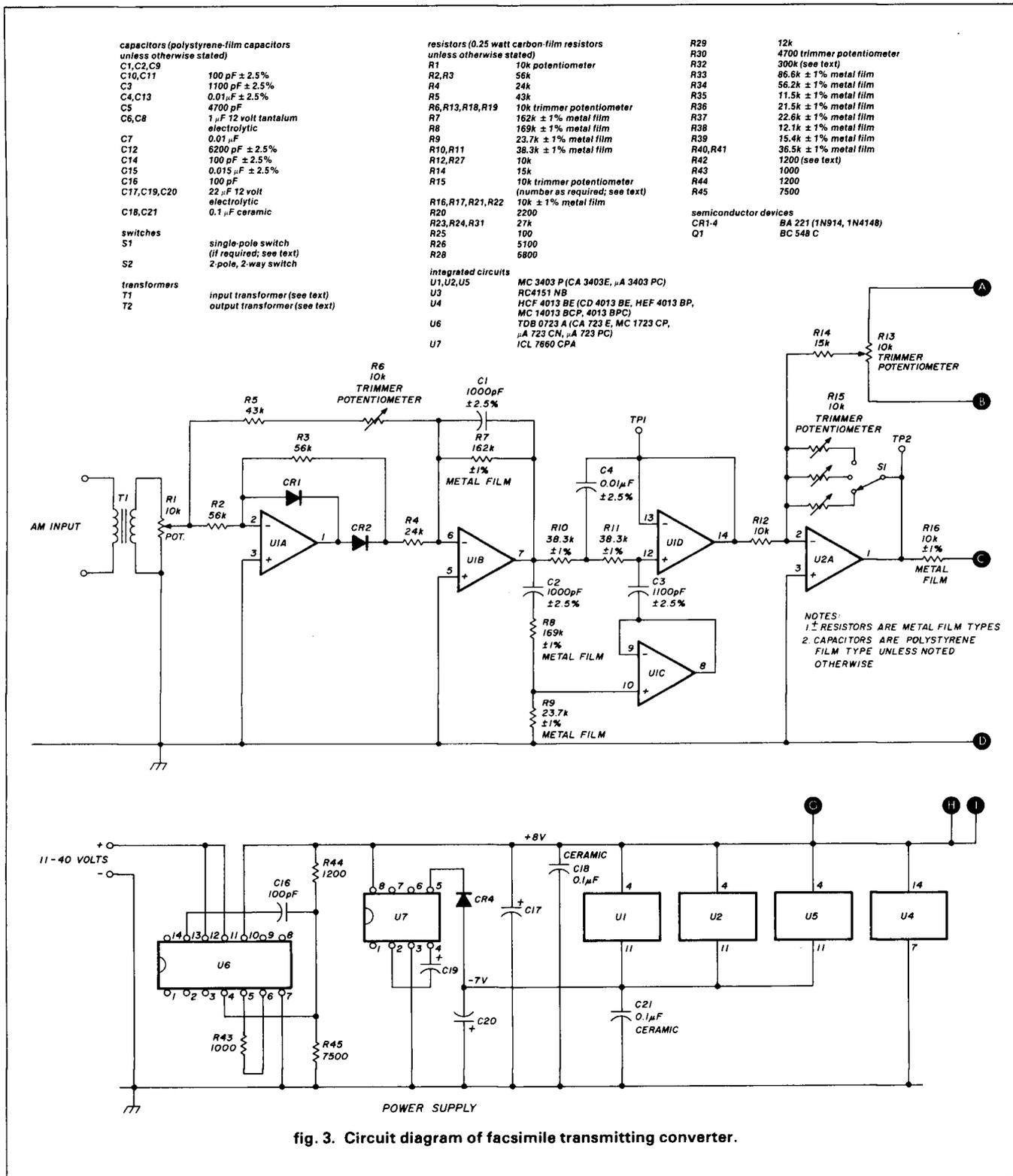
fig. 3. Circuit diagram of facsimile transmitting converter.
