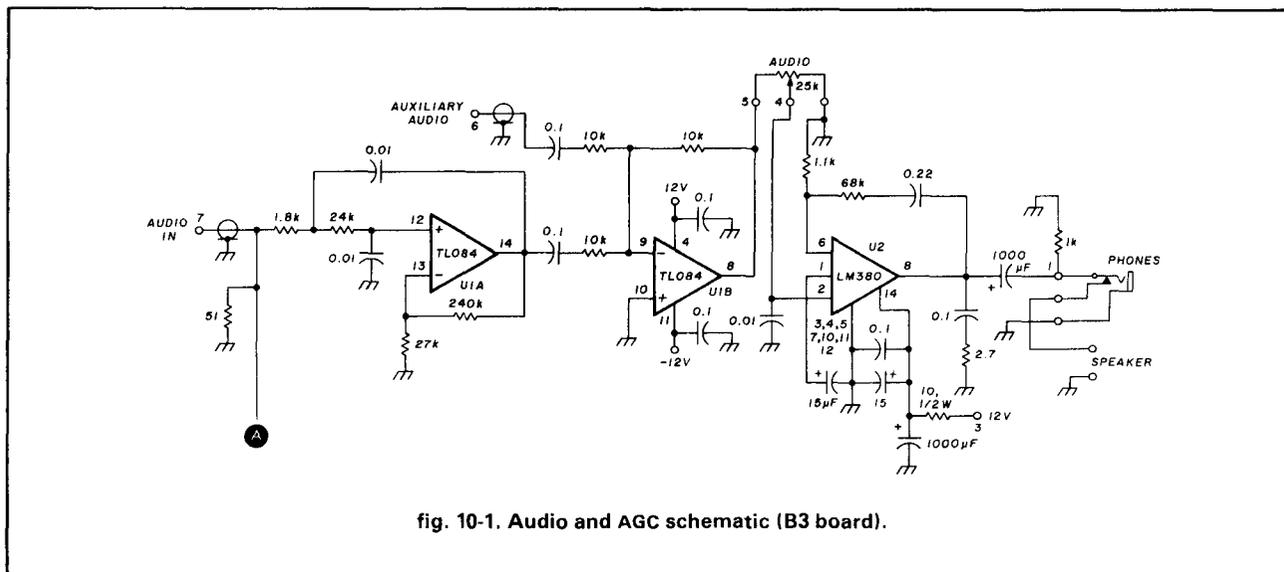
fig. 10-1. Audio and AGC schematic (B3 board).
