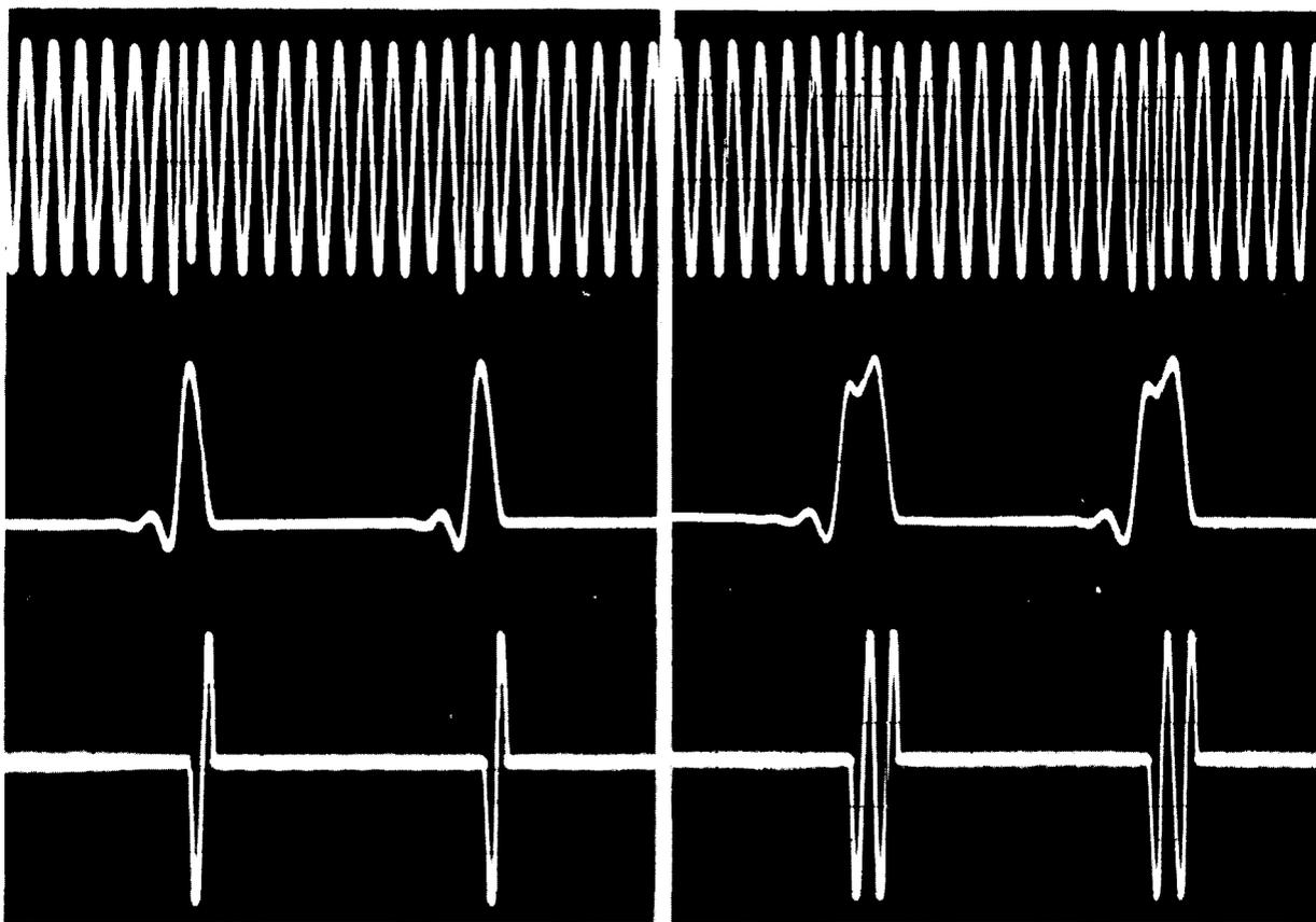
fig. 10. Overall response (bottom) to burst-modulated 1800-Hz sine wave (top) applied to converter input, producing at TP3 a video signal (center) alternating between  $-1500$  mV and  $-2300$  mV. Burst duration  $1100 \mu\text{s}$  (left) and  $555 \mu\text{s}$  (right).
