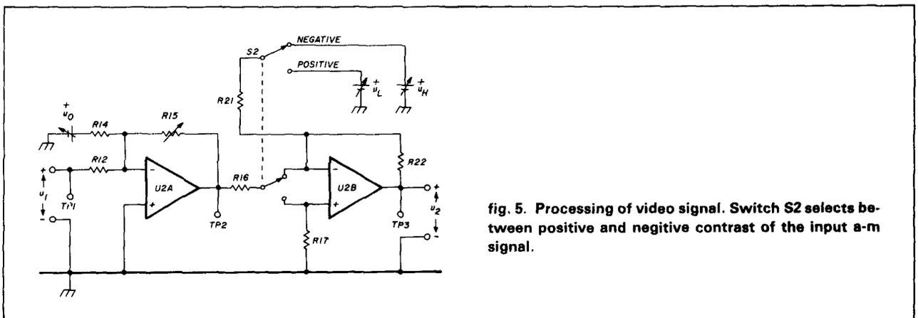
fig. 5. Processing of video signal. Switch S2 selects between positive and negative contrast of the input a-m signal.
