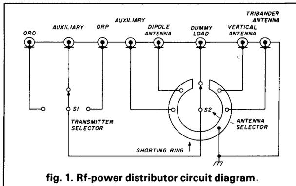
fig. 1. Rf-power distributor circuit diagram.
