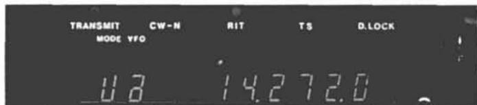
**Broadbanded solid state transceiver operation** on the 9 amateur HF bands — Readout of mode in use and VFO — Status LEDs for push button functions.
