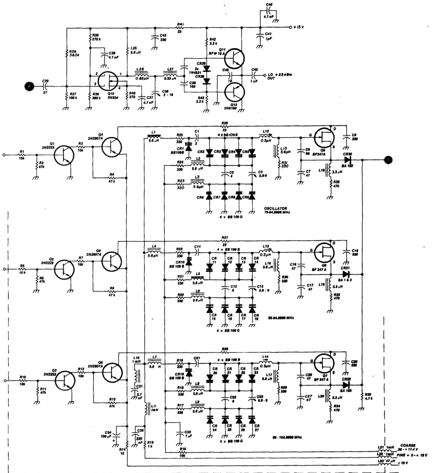
fig. 12. Schematic diagram of three low-noise VCOs with coarse and fine tuning input, select circuits, and 23-dBm post amplifier, recommended for shortwave receivers.
