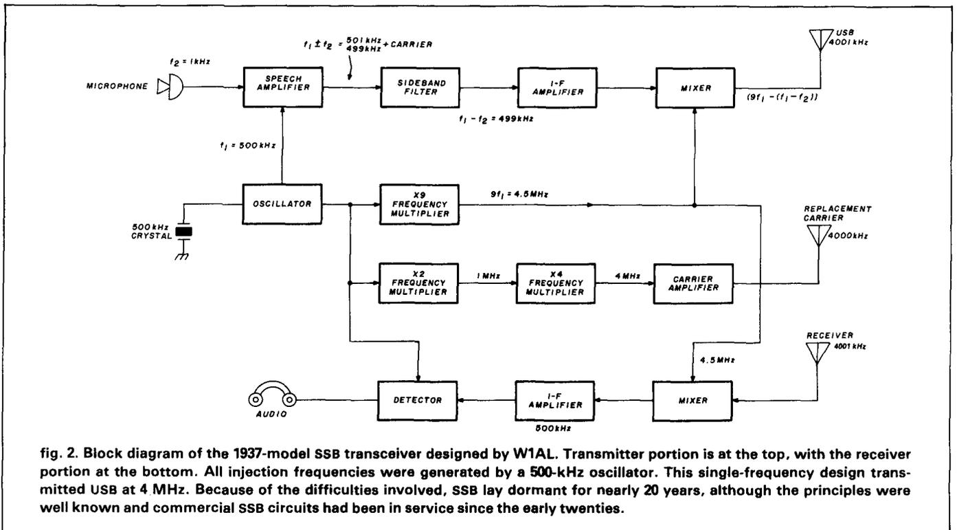
fig. 2. Block diagram of the 1937-model SSB transceiver designed by W1AL. Transmitter portion is at the top, with the receiver portion at the bottom. All injection frequencies were generated by a 500-kHz oscillator. This single-frequency design transmitted USB at 4 MHz. Because of the difficulties involved, SSB lay dormant for nearly 20 years, although the principles were well known and commercial SSB circuits had been in service since the early twenties.
