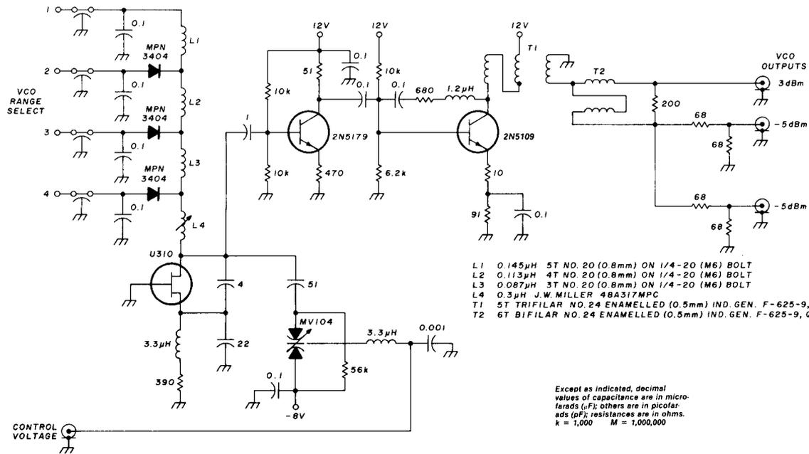
fig. 11. 45 to 75-MHz VCO schematic (part of M7 module). Unit uses a grounded-gate U310 FET in a Colpitts circuit. One of four ranges may be selected by applying 8 volts to a range-select input. Tuning is by an MV104 varactor.
