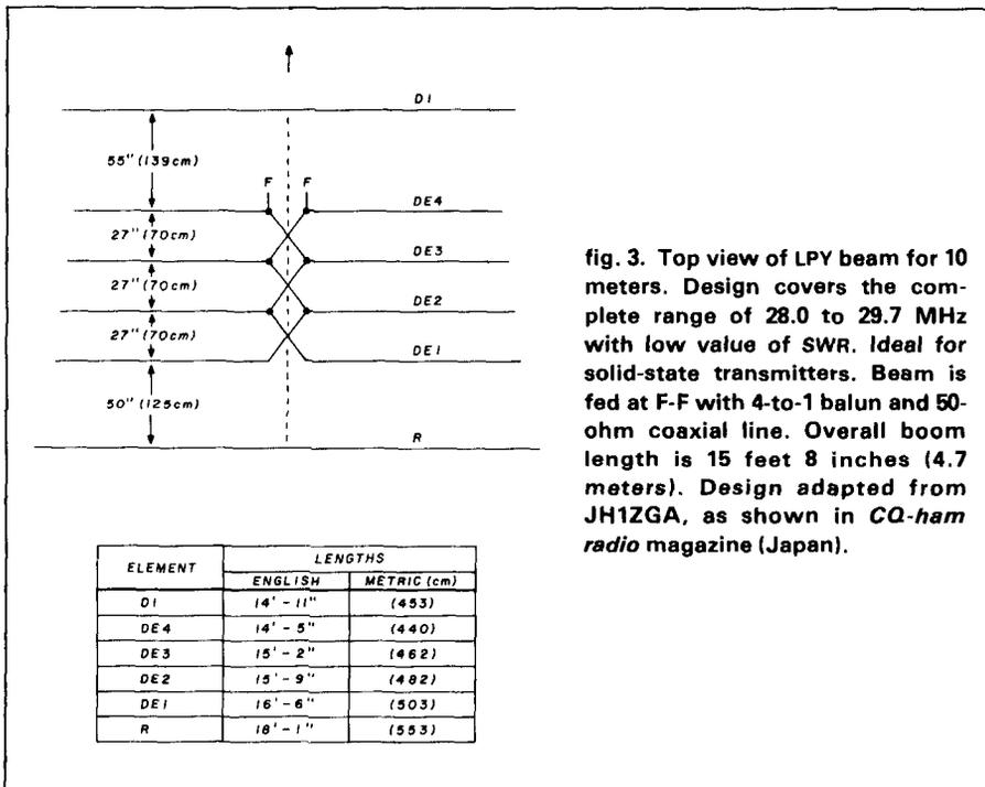
fig. 3. Top view of LPY beam for 10 meters. Design covers the complete range of 28.0 to 29.7 MHz with low value of SWR. Ideal for solid-state transmitters. Beam is fed at F-F with 4-to-1 balun and 50-ohm coaxial line. Overall boom length is 15 feet 8 inches (4.7 meters). Design adapted from JH1ZGA, as shown in *CQ-ham radio* magazine (Japan).
