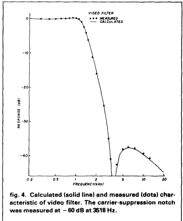
fig. 4. Calculated (solid line) and measured (dots) characteristic of video filter. The carrier-suppression notch was measured at  $-60 \text{ dB}$  at  $3518 \text{ Hz}$ .
