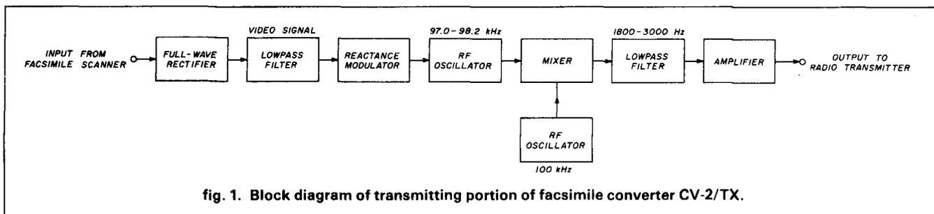
fig. 1. Block diagram of transmitting portion of facsimile converter CV-2/TX.
