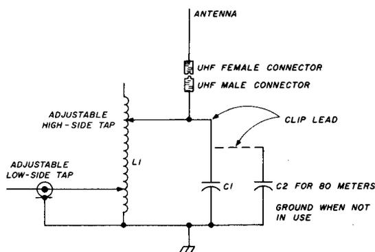
fig. 4. Tuning network is completely adjustable. The inductance is made of 15 turns of B&W No. 3033 coil stock (15  $\mu$ H); capacitor is made of RG-8/U coax cable as described in the text. In this arrangement C1 is 38.1 pF. System resonates at 7.15 MHz.
