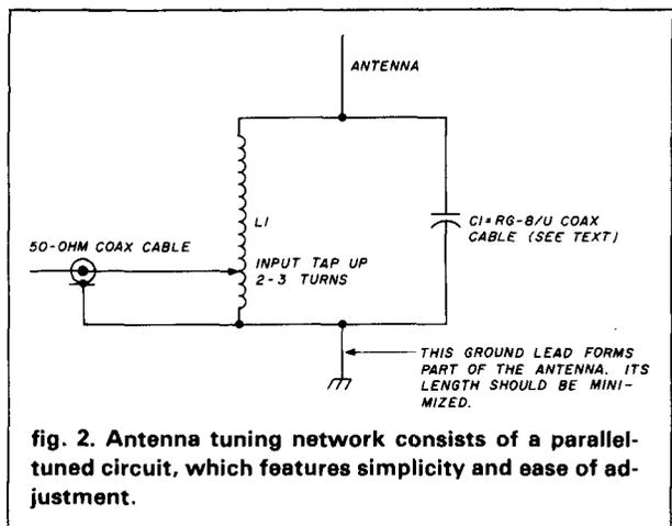
fig. 2. Antenna tuning network consists of a parallel-tuned circuit, which features simplicity and ease of adjustment.
