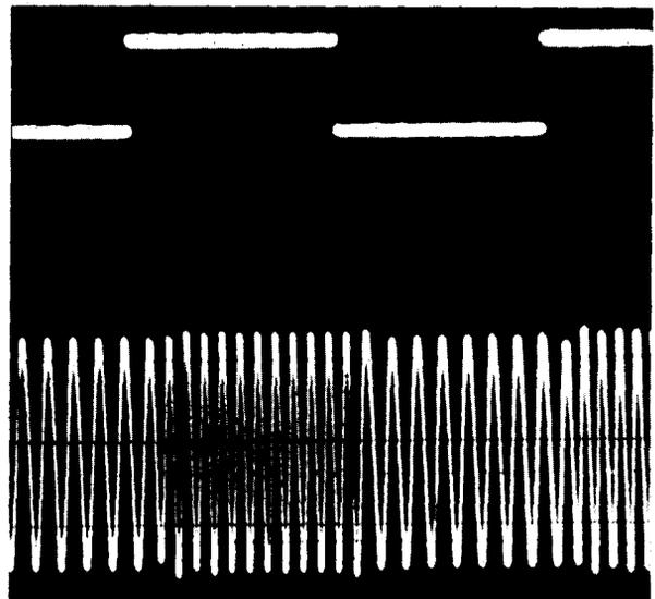
fig. 9. Output signal of 1500 Hz and 2300 Hz (bottom) produced by 100-Hz square-wave train (top) applied to input of video filter.
