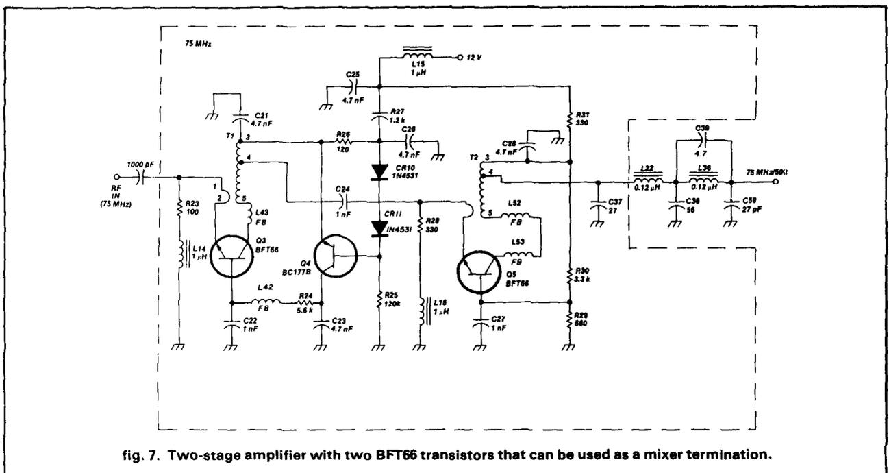
fig. 7. Two-stage amplifier with two BFT66 transistors that can be used as a mixer termination.
