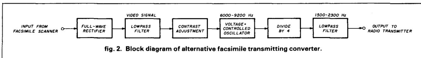
fig. 2. Block diagram of alternative facsimile transmitting converter.
