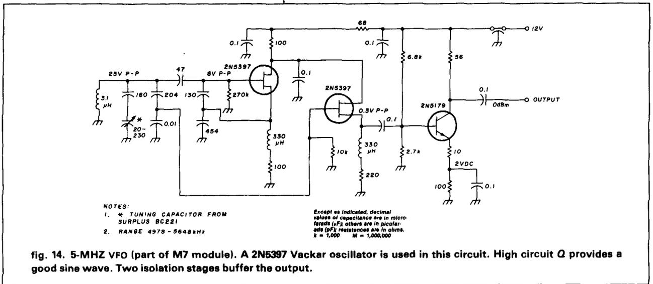
The VFO has been very satisfactory in operation; however, I could have used heavier material than a minibox, because a shift of 100 Hz is noticeable if the receiver is turned upside down while listening to a CW signal. Flexing of the tuned circuit components causes this problem.
