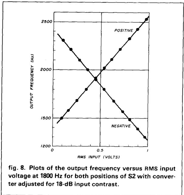
fig. 8. Plots of the output frequency versus RMS input voltage at 1800 Hz for both positions of S2 with converter adjusted for 18-dB input contrast.
