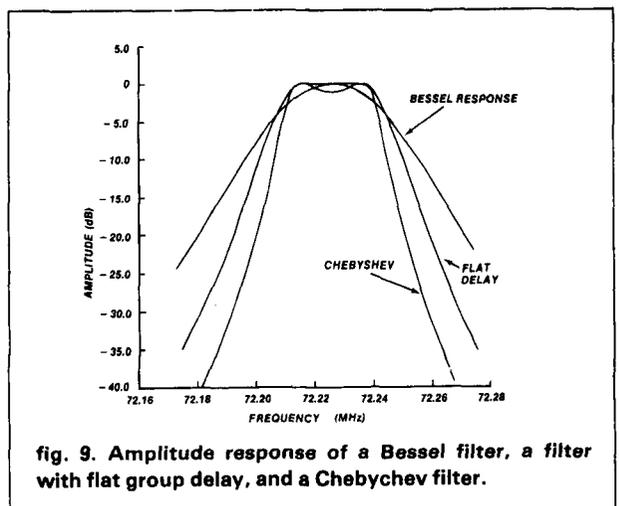
fig. 9. Amplitude response of a Bessel filter, a filter with flat group delay, and a Chebyshev filter.
