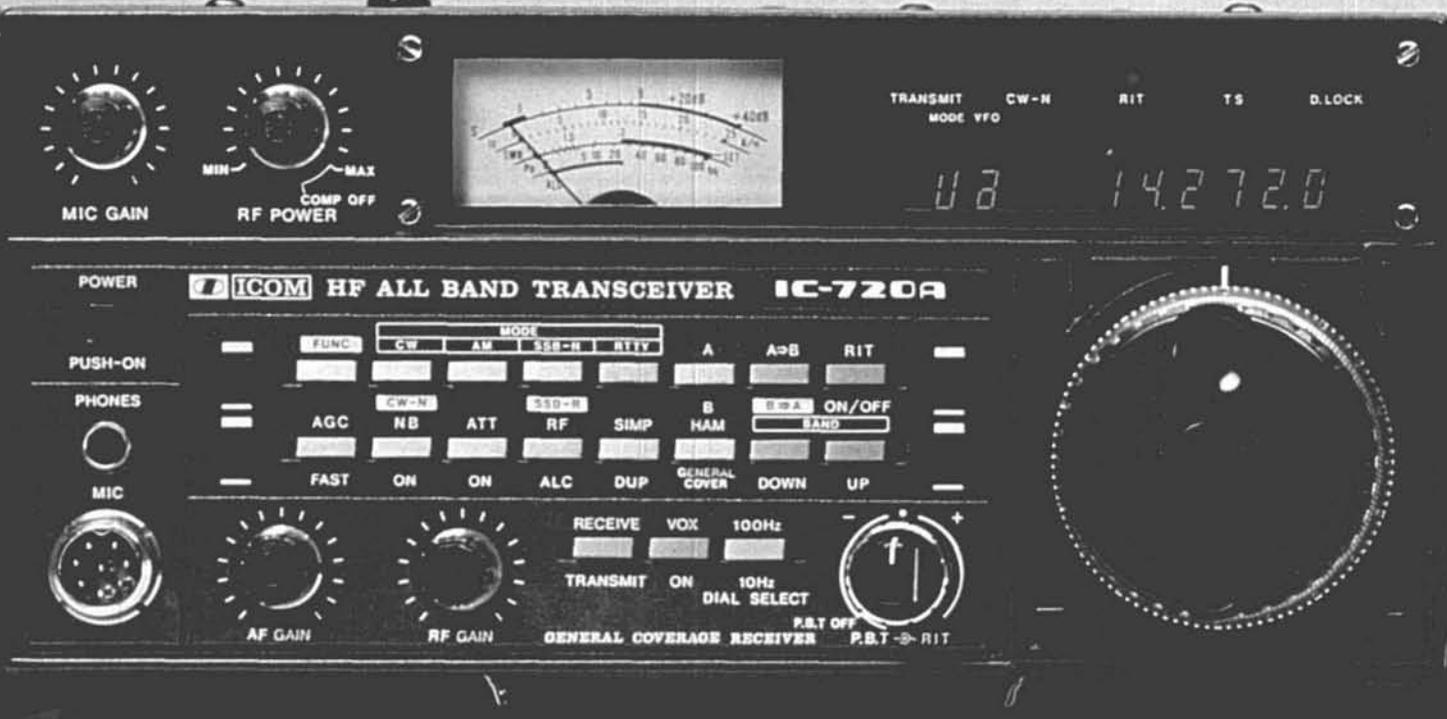
**Multi mode operation** includes CW/AM/SSB/RTTY — Normally used side band selected automatically.
