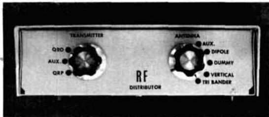
Front view and rear view of the home made rf-power distributor.
