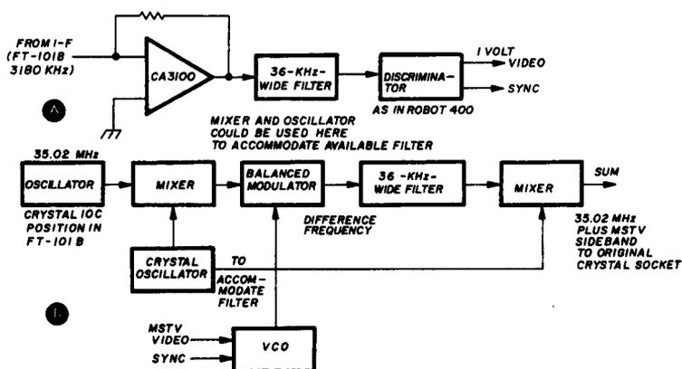
fig. 2. Block diagram for the proposed modifications to an FT-101 or similar transceiver. Conversions for receiver and transmitter sections are shown in A and B respectively.
