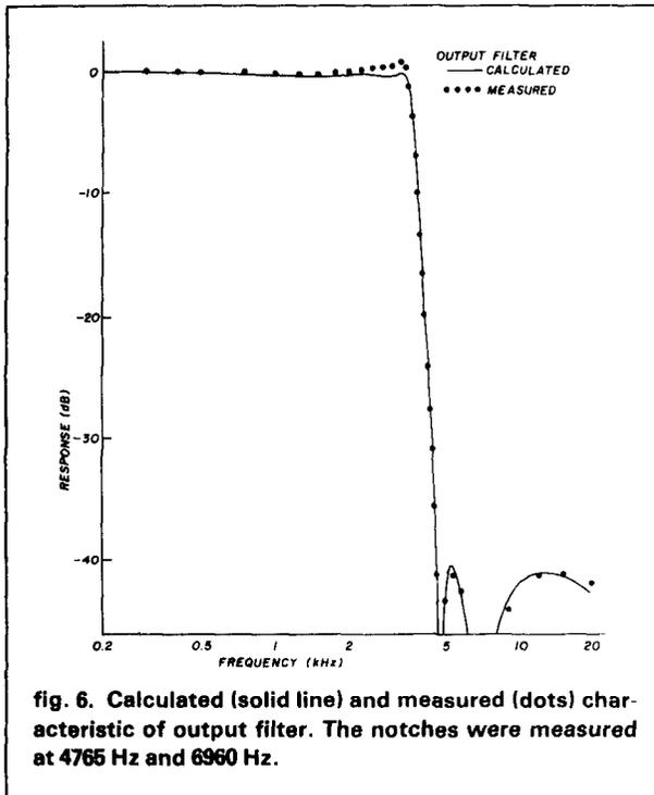
fig. 6. Calculated (solid line) and measured (dots) characteristic of output filter. The notches were measured at 4765 Hz and 6960 Hz.
