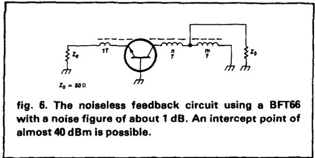
fig. 6. The noiseless feedback circuit using a BFT66 with a noise figure of about 1 dB. An intercept point of almost 40 dBm is possible.
